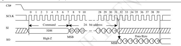
Figure 9-61 Read Block Lock Status (SPI)
