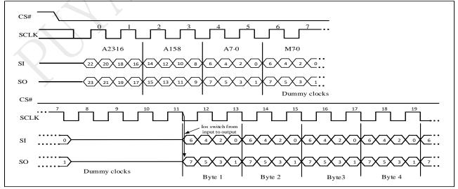
Figure 9-21a DTR 2IO Continuous Read Sequence (SPI, M5-4 = (1,0))
