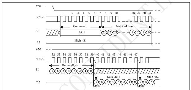
Figure 9-68 Read Serial Flash Discoverable Parameter (RDSFDP) Sequence (SPI)
