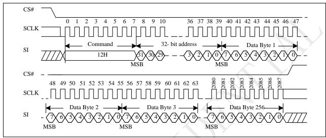
Figure 9-41 Page Program with 4-Byte Address Sequence (SPI)
