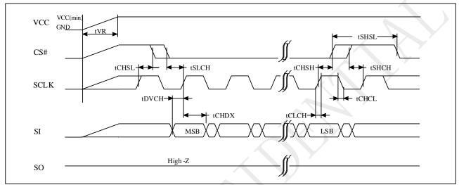
Figure 5-8 AC Timing at Device Power-Up
