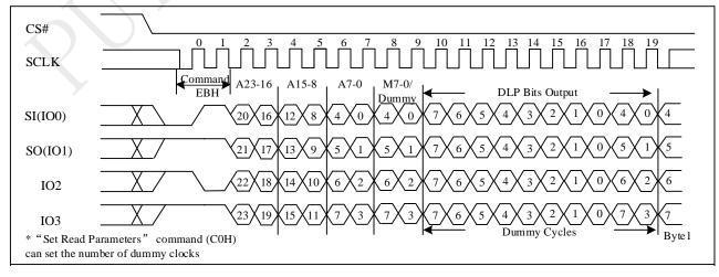
Figure 9-30f 4IO Read with DLP bits output Sequence (QPI)
