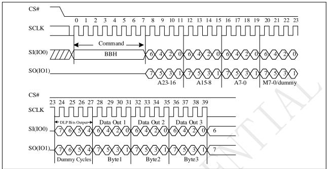
Note: The DLP bit is also valid for 4-byte BBH and BCH instruction Figure 9-30e 4IO Read with DLP bits output Sequence (SPI)
