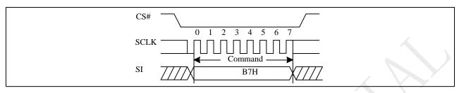
Figure 9-11a Enter 4-Byte Address Mode Sequence (QPI)
