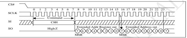
Figure 9-9a Read Extended Address Register Sequence (QPI)
