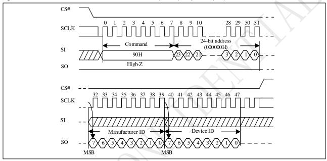
Figure 9-51 Read Electronic Manufacturer & Device ID (REMS) Sequence (SPI)
